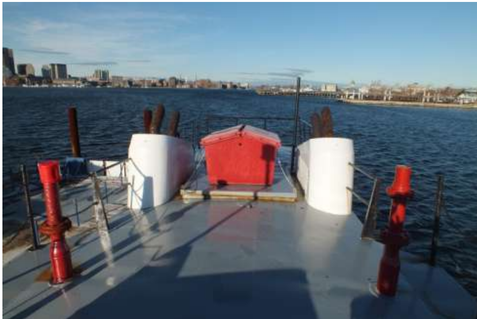
Upper deck, looking aft. Notice cut off fire main risers.
