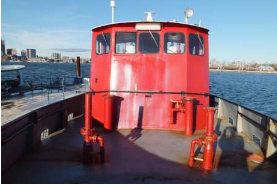
Foredeck, looking aft. Notice steel risers where fire monitors have been removed.
