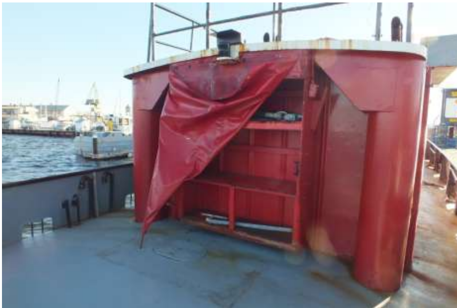
Aft end of doghouse, showing shelving and fabric cover for hand tools.
