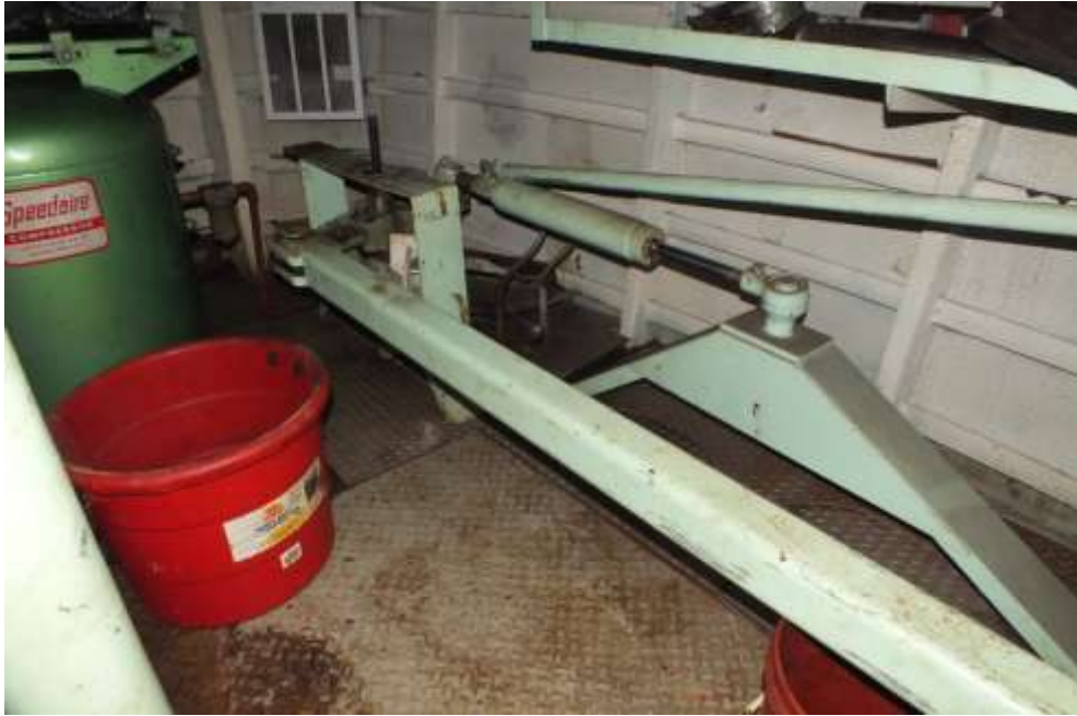
Starboard side of lazarette, showing starboard rudder post and steering gear assembly.
